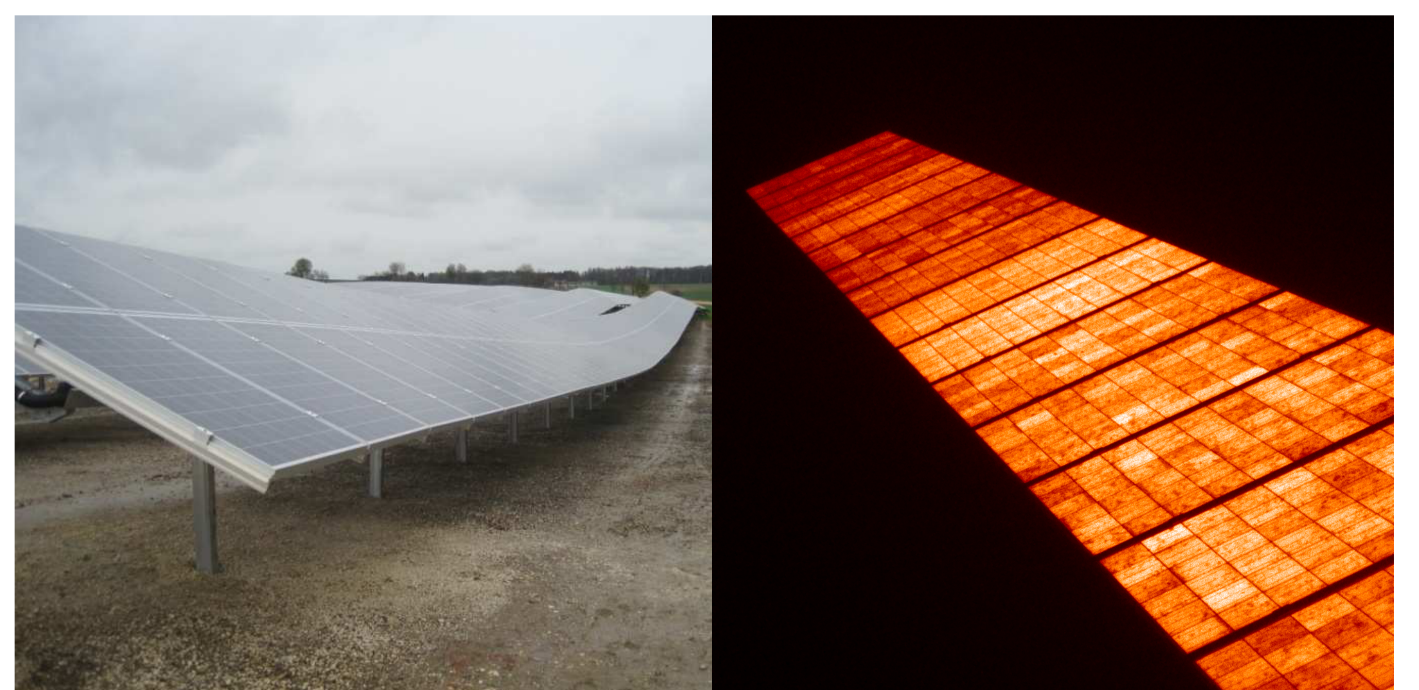
Left: Visible Image of Solar module string, right: EL Image measured under night sky using a line-powered 10KW supply
