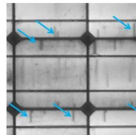
Fig. 9 Contact finger interruptions in a mono-crystalline silicon cell
