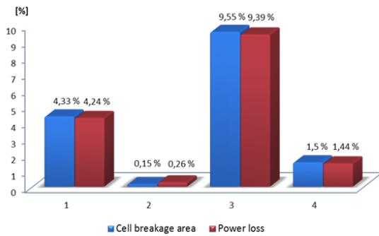
Fig. 5 Correlation between cell breakage area and power loss
