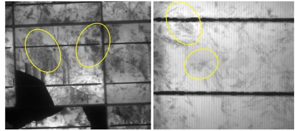
Fig. 7 Crystal inhomogeneities in crystalline silicon cells
