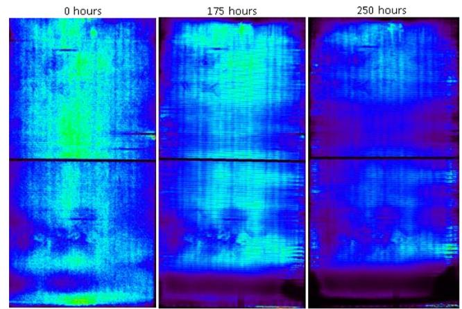
Fig. 11 Progression of the TCO corrosion in a thin film CdTe module
