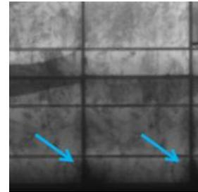
Fig. 8 Defective edge isolation
