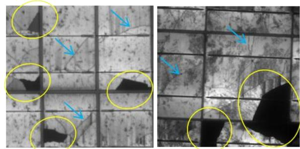
Fig. 4 Cracks and breakages in crystalline silicon cells
