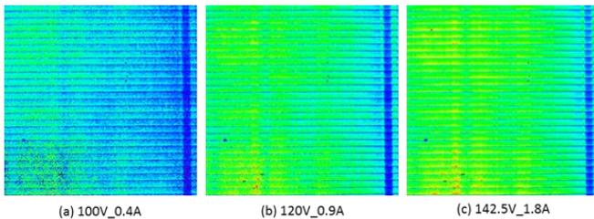
Fig. 2. Effect of operating voltage and current on image quality
